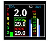
The two boxes, green and red, with 29.0 in the center indicate the current firing angle of the right (top/green) and left (bottom/red) ignitions. This number will change based on the RPM, manifold pressure, and timing configuration.
